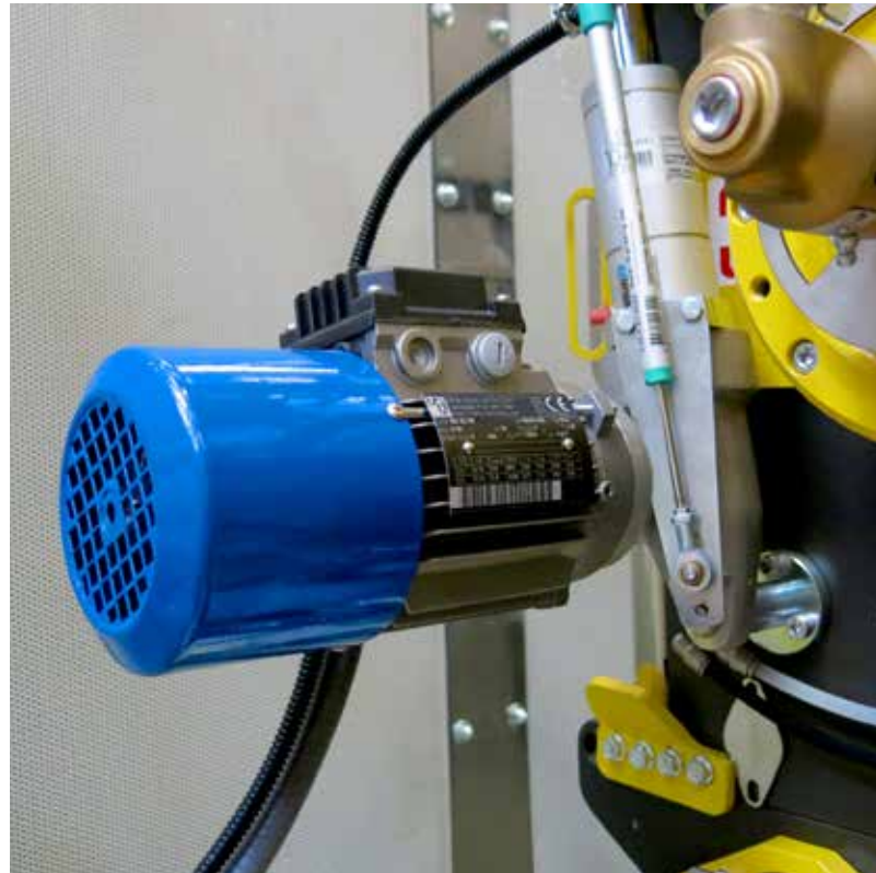
Roots gap control with linear motor
